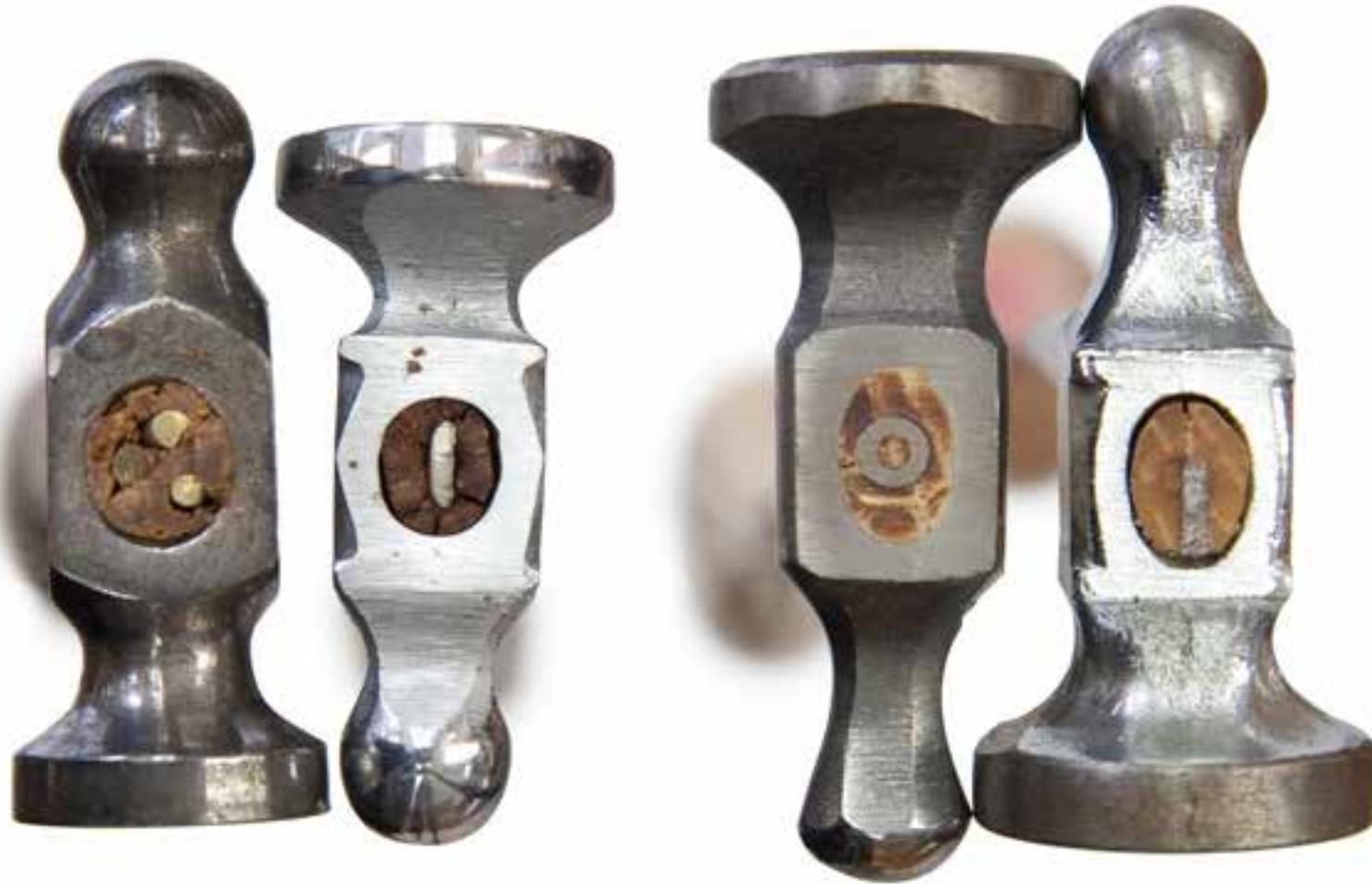
**Top view of the hammer heads, showing the sockets. The cheap ones are on the left this time.**
